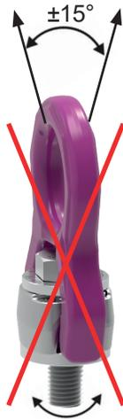
Pic. 11: Prohibited rotation under load in the direction of the bolt axle.
