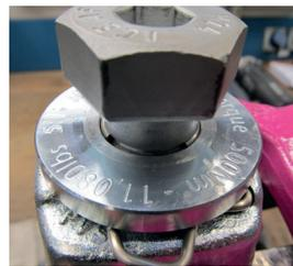
Pic. 14: Circlip fully positioned in the recess of the countersink
