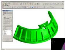
DIMENSIONAL CONTROL performed on our Coordinate Measuring Machine through our dedicated Computer Aided Quality Control software (math.3D model vs. prototype) Component: Bracket for space application Material: Inconel 718 - AMS5662 Rough bar dim. & weight: Ø 270 x 470 mm (220 kg) Finished part weight: 5 kg approx. Features: 5 axes sculpturing, before and after aging condition
