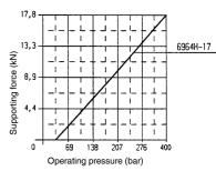
0,004 mm/kN elastic change in length under load
