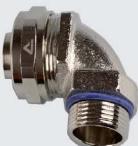
Pg 90° fitting, compact, male, nickel plated brass (incl. connection set)
