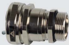
ISO cable-hose fitting, compact, male, double seal acc. EN 45545-2, HL1 / HL2 / HL 3, table R22 and R23 (incl. connection set)
