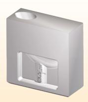
For tunnel gating of medium-to-large components. Supports contouring to a depth of 11,5 mm. Suitable for gate diameters up to 3,5 mm and shot weights up to 1,200 g per insert. The Maxiflow range can be used to process all common plastics, including reinforced types.
