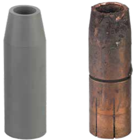
Gas nozzle: VOLCERA after 100 shifts in continuous operation and copper after 1 shift
