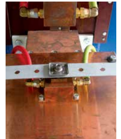
Sheet and projection weld nut in the welding machine
