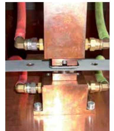
Welding process in the projection weld nut machine
