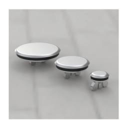
**Description:** Seal extra pushbutton holes, conduit openings and knockout openings against dust, dirt, oil and water with Hoffman Hole-Sealers. Seals will cover any size or shape of hole from 5mm diameter to maximum diameter shown in table. Can be used on enclosure walls up 8-mm thick.
