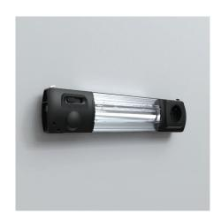
**Description:** LED enclosure light specially designed for nVent HOFFMAN enclosures. Fast and tool-free assembly thanks to a latching hook system designed to fit the 25mm hole pattern on nVent HOFFMAN enclosures. May be fitted horizontally or vertically.
