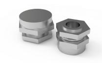
**Description:** Combination of drainage and breathing elements especially for use in potentially explosive atmosphere. Type of protection: Flameproof (Ex d). Thread length: 16 mm. To be installed in a threaded hole. Position at the lowest point of an enclosure to ensure optimal draining of any moisture.
