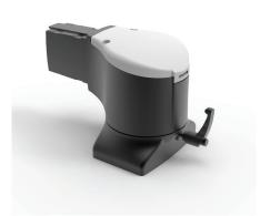
**Additional information:** The flange elbow coupling attaches directly to the enclosure for applications where a vertical tube is not required. It enables the enclosure to rotate 300 degrees and can be locked into a given position. The flange elbow coupling has a safety stop and maintenance-free bearings. Die-cast aluminum construction. Includes installation instructions, gaskets, tube setscrews and enclosure mounting hardware.
