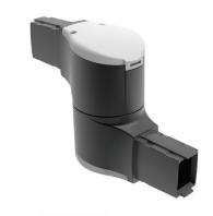
**Additional information:** Use an intermediate joint to join two horizontal tubes together for a longer length. The arm can be rotated 300 degrees. Includes safety stop and maintenance-free bearings. Die-cast aluminum construction. Includes installation instructions, gaskets, and tube setscrews. Use of the intermediate joint reduces the system load rating capacity to 146 lb. (66 kg) at 3.3 ft. (1 m).
