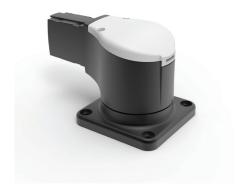
**Additional information:** The set-up joint mounts the suspension system to a horizontal surface. The arm can be rotated 300 degrees. Includes a safety stop and maintenance-free bearings. Die-cast aluminum construction. Includes installation instructions, gaskets, and tube setscrews. Surface mounting hardware is not provided.
