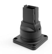
**Additional information:** The rotatable base bracket allows the entire suspension system to rotate at the point of attachment on a horizontal surface. The arm can be rotated 300 degrees. Includes a safety stop and maintenance-free bearings. Die-cast aluminum construction. Includes installation instructions, gaskets, and tube setscrews. Surface mounting hardware is not provided.
