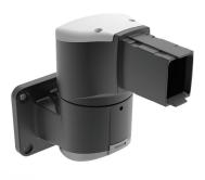
**Additional information:** The horizontal wall joint mounts the suspension system to a vertical surface, allowing the tube to extend horizontally. The arm can be rotated 300 degrees. Includes a safety stop and maintenance-free bearings. Die-cast aluminum construction. Includes installation instructions, gaskets, and tube setscrews. Surface mounting hardware is not provided.
