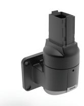
**Additional information:** The vertical wall joint mounts the suspension system to a vertical surface, allowing the tube to extend vertically. The arm can be rotated 300 degrees. Includes a safety stop and maintenance-free bearings. Die-cast aluminum construction. Includes installation instructions, gaskets, and tube setscrews. Surface mounting hardware is not provided.
