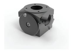
**Additional information:** Angled Adapter must be used in conjunction with a coupling (not compatible with S2MFC48). The enclosure angle can be adjusted forward or backward up to 30 degrees. RAL 9005 black finish. Die-cast aluminum construction. Includes installation instructions, gasket and enclosure mounting hardware. Maximum load bearing capacity is 67 lb. (30.4 kg).
