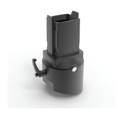
**Additional information:** Use Angled Coupling Tilted Backward to mount enclosure at a 15-degree backward angle. The enclosure can be rotated 300 degrees and locked in position. Includes safety stop and maintenance-free bearing. RAL 9005 black finish. Die-cast aluminum construction. Includes installation instructions, gaskets, tube setscrews and enclosure mounting hardware.
