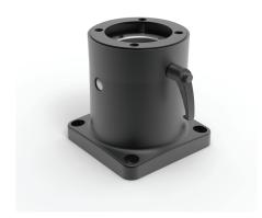
**Additional information:** Base Coupling attaches the enclosure directly to a horizontal surface. The enclosure can be rotated 300 degrees and locked in position. Includes safety stop and maintenance-free bearing. RAL 9005 black finish. Diecast aluminum construction. Includes installation instructions, gaskets and enclosure mounting hardware. Surface mounting hardware is not provided.
