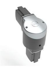
**Additional information:** Rotatable elbow provides a 90-degree bend in the suspension system and allows the vertical tube to rotate 300 degrees. Includes safety stop and maintenance-free bearing. RAL 9005 black finish. Die-cast aluminum construction. Includes removable cable access cover, installation instructions, gaskets and tube setscrews.
