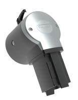
**Additional information:** Flange Elbow Coupling attaches directly to the enclosure for applications where a vertical tube is not required. Enables the enclosure to be rotated 300 degrees and locked in position. Includes safety stop and maintenance-free bearing. RAL 9005 black finish. Die-cast aluminum construction. Includes cable access cover, installation instructions, gaskets, tube setscrews and enclosure mounting hardware.
