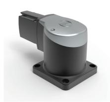
**Additional information:** Set-Up Joint mounts suspension system to a horizontal surface. The arm can be rotated or turned 300 degrees. Includes safety stop and maintenance-free bearing. RAL 9005 black finish. Die-cast aluminum construction. Includes removable cable access cover, installation instructions, gaskets and tube setscrews. Surface mounting hardware is not provided.
