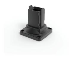
**Additional information:** Wall Flange allows for fixed positioning on a horizontal or vertical surface when rotation is not needed. RAL 9005 black finish. Diecast aluminum construction. Includes installation instructions, gaskets and tube setscrews. Surface mounting hardware is not provided.
