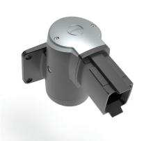
**Additional information:** Horizontal Wall Joint mounts suspension system to vertical surface, allowing tube to extend horizontally. The arm can be rotated or turned 300 degrees. Includes safety stop and maintenance-free bearing. RAL 9005 black finish. Diecast aluminum construction. Includes two removable cable access covers, installation instructions, gaskets and tube setscrews. Surface mounting is hardware not provided.
