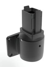
**Additional information:** Vertical Wall Joint mounts suspension system to vertical surface and allows tube to extend vertically. Enables the arm to be rotated or turned 300 degrees. Includes safety stop and maintenance-free bearing. RAL 9005 black finish. Die-cast aluminum construction. Includes removable cable access cover, installation instructions, gaskets and tube setscrews. Surface mounting hardware is not provided.
