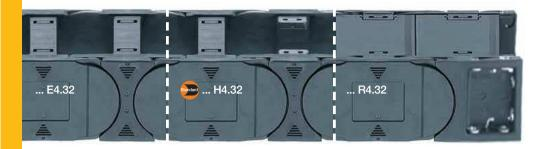
e-chains® | Series E4.32 | Crossbars every link (crossbars removable along the inner and outer radius) e-chains® Series H4.32 Crossbars every 2nd link (crossbars removable along the inner and outer radius) e-tubes Series R4.32 Fully enclosed (lids openable along the outer radius, from one side)
