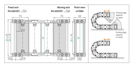
KMA pivoting | Recommended for unsupported and gliding applications Recommended for vertical hanging and standing applications KMA locking
