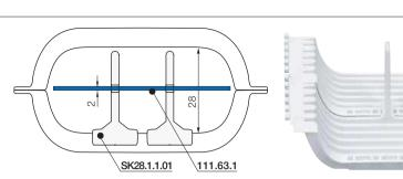
e-skin separators should be fitted every 112mm onto the connection points!
