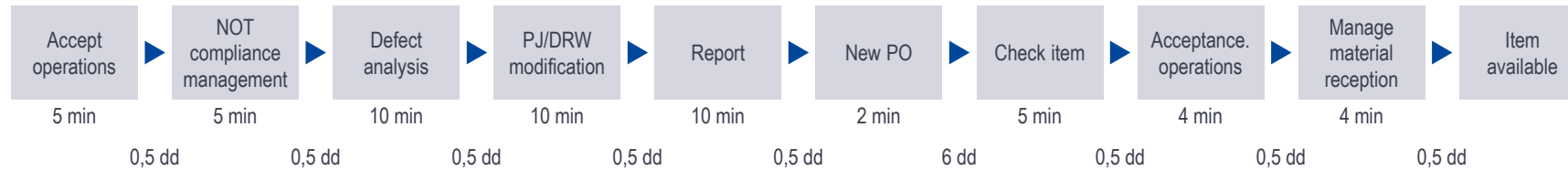
AVERAGE MINUTES OF MAN WORKING TIME AND DAYS OF DELAY RELATED TO A NON CONFIRMITY
