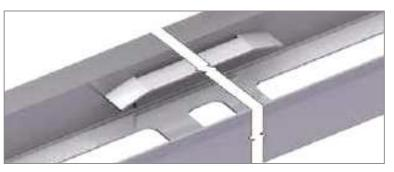
A special slide support can be adhered to reduce sliding resistance and abrasion between cable carrier and support. We recommend the use of special slide supports for velocities > 0.5 m/s and for frequent move cycles.
