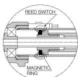
The magnetic field of the ring fixed on the nut activates the reed contact of the switch locked on the protective tube with a clamp.
