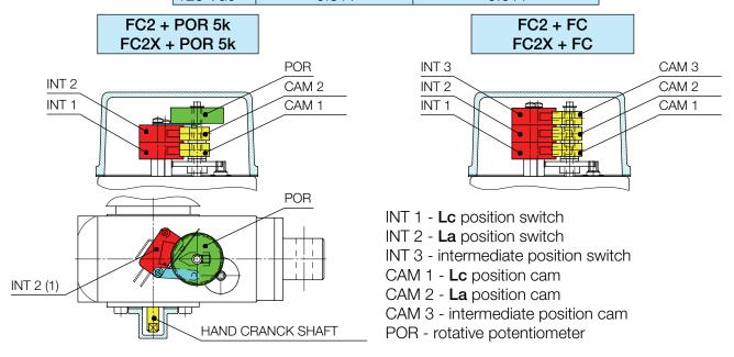
Lc = actuator retracted length, La = Lc + Stroke - actuator extended length
