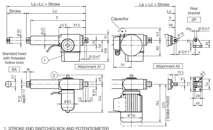
2. MOTOR SHAFT EXTENSION for: Emergency manual activation Stroke end switches and potentiometer adjustment
