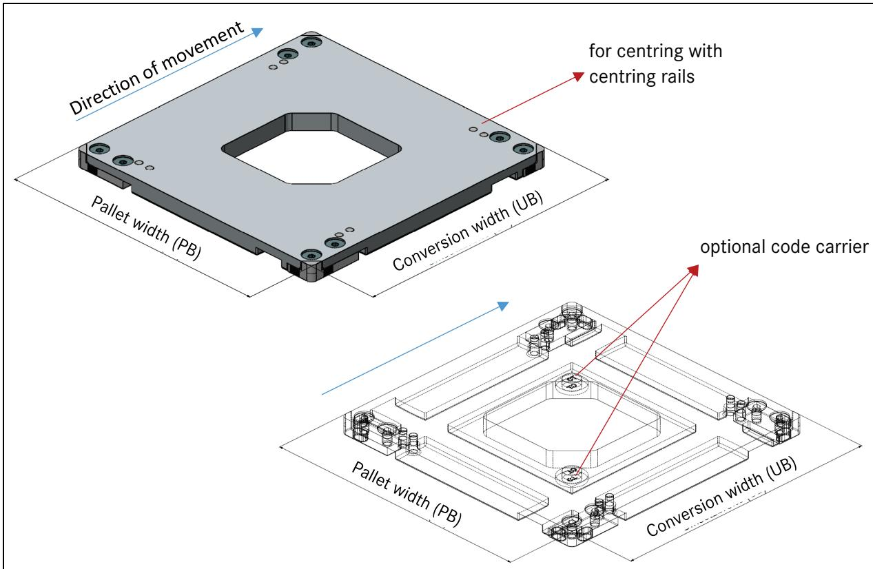
The workpiece carrier (WT) has the function of optimally guiding your product on the transfer system through the assembly. It rests on the two conveyor belts of the belt element and is driven by them. Sliding strips mounted laterally in the belt profile guide the workpiece carrier. The centring pins allow the WT to be centred with the help of centring rails.
