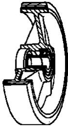
**Tread:** “TR” polyurethane tread, hardness 95+/-3 Shore A; excellent rolling resistance and elasticity, highly resistant to wear and to tearing.
