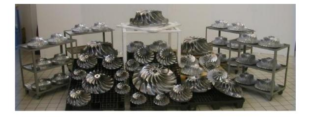
Thanks to the smart balancing between the long experience of some of its specialists in the aeronautical domain and the enthusiasm of a young team of engineers. APR has grown with the <u>passion</u> for five axes simultaneous machining dedicated to impellers manufacturing.
