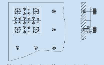
This type of sandwich plate is ideal for mounting adapter plates with locating screws
